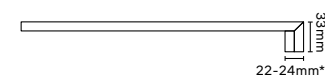
step tread "L" corner . nez de marche "L" angle ecke stufenplatte "L" . degrau "L" canto
